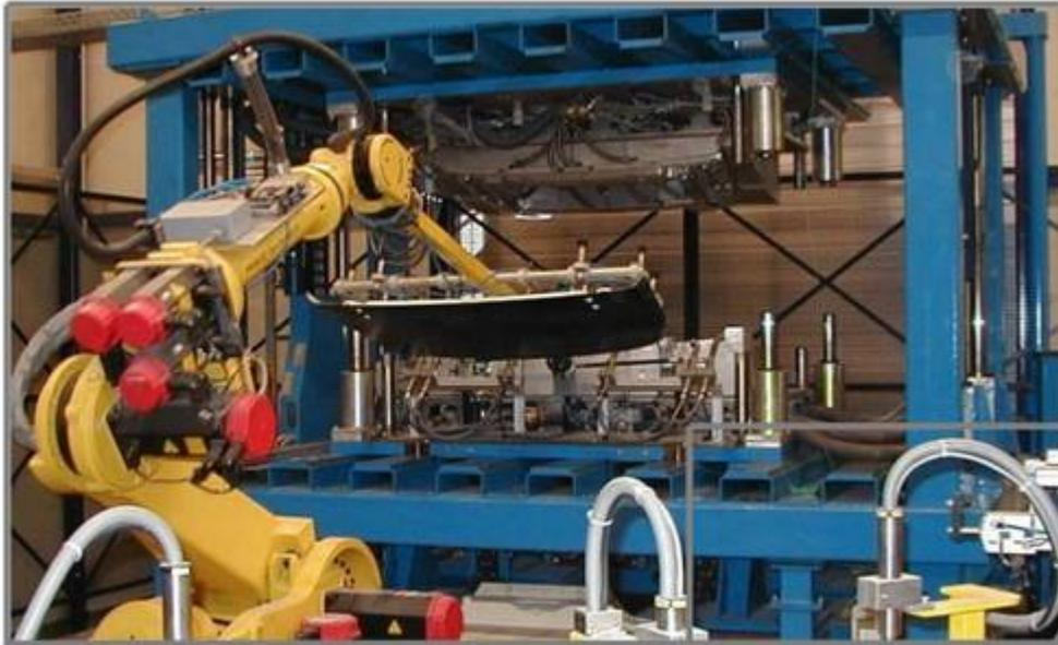
Heated Fixture for Bonding an Automotive trunklid
