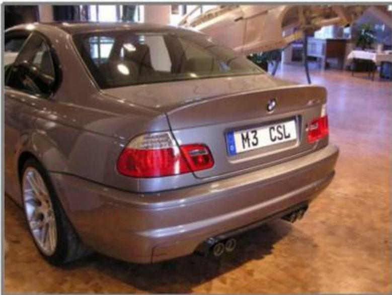
Trunk Lid of BMW's M3 CSL consisting of two bonded SMC parts
