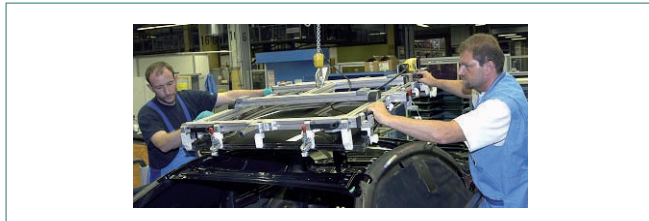
Fig. 7: BMW M3 CSL - Bonding the CFRP roof to the body [11]
