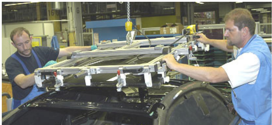
Fig. 10: BMW M3 CSL – Bonding the CFRP Roof to the Body [11]
